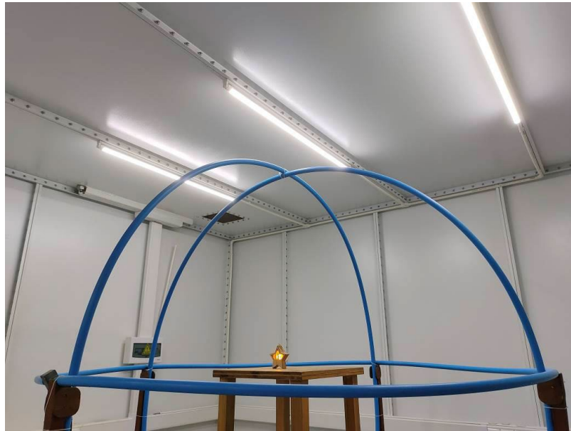
EN IEC 55015 RADIATED ELECTROMAGNETIC DISTURBANCE TEST SETUP
