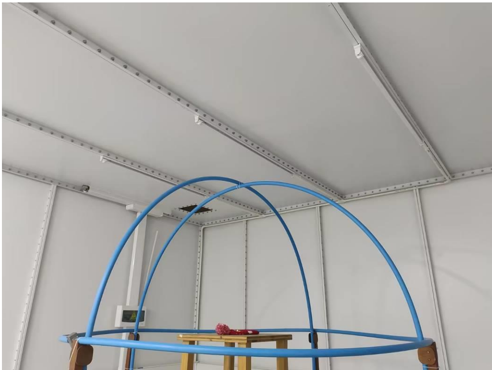
EN IEC 55015 RADIATED ELECTROMAGNETIC DISTURBANCE TEST SETUP
