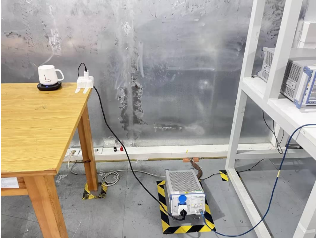
Photo of Power Line Conducted Measurement
