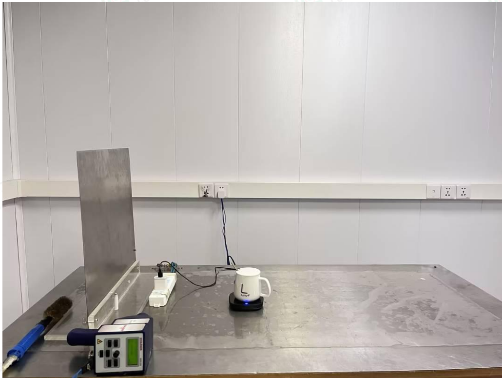
Photo of Electrostatic Discharge Test
