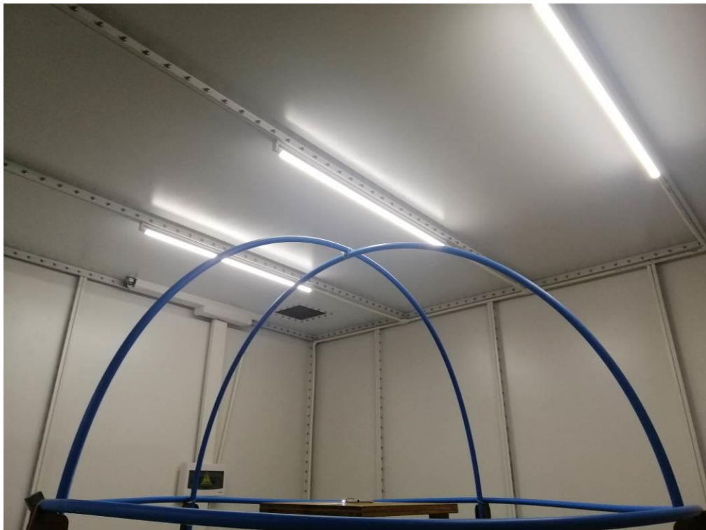
EN IEC 55015 RADIATED ELECTROMAGNETIC DISTURBANCE TEST SETUP
