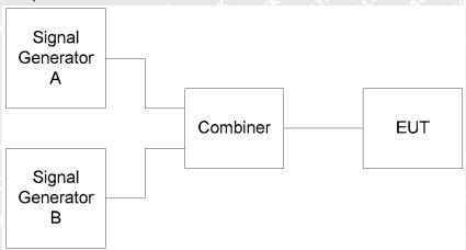
Two signal generators A and B shall be connected to the receiver via a combining network to the receiver antenna connector.
