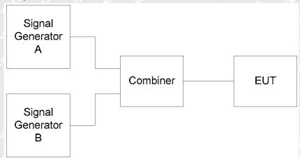
Two signal generators A and B shall be connected to the receiver via a combining network to the receiver antenna connector.
