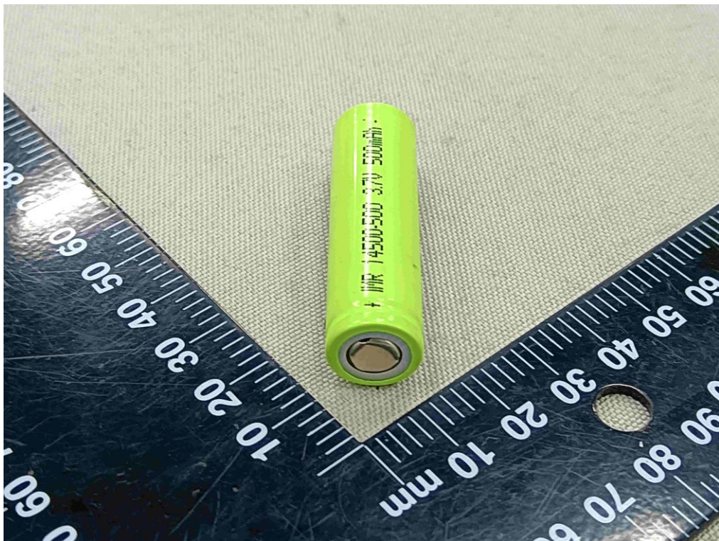
Figure 4 Side view of cell (model: IMR14500-500mAh)
