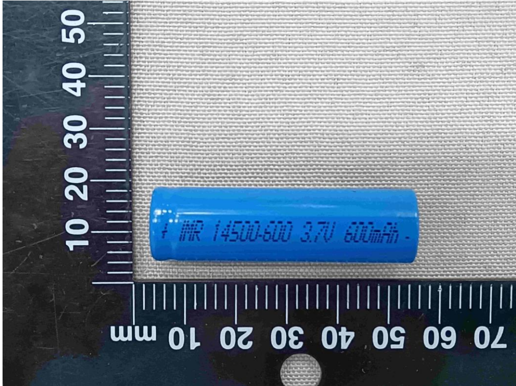
Figure 1 Front view of cell (model: IMR14500-600mAh)
