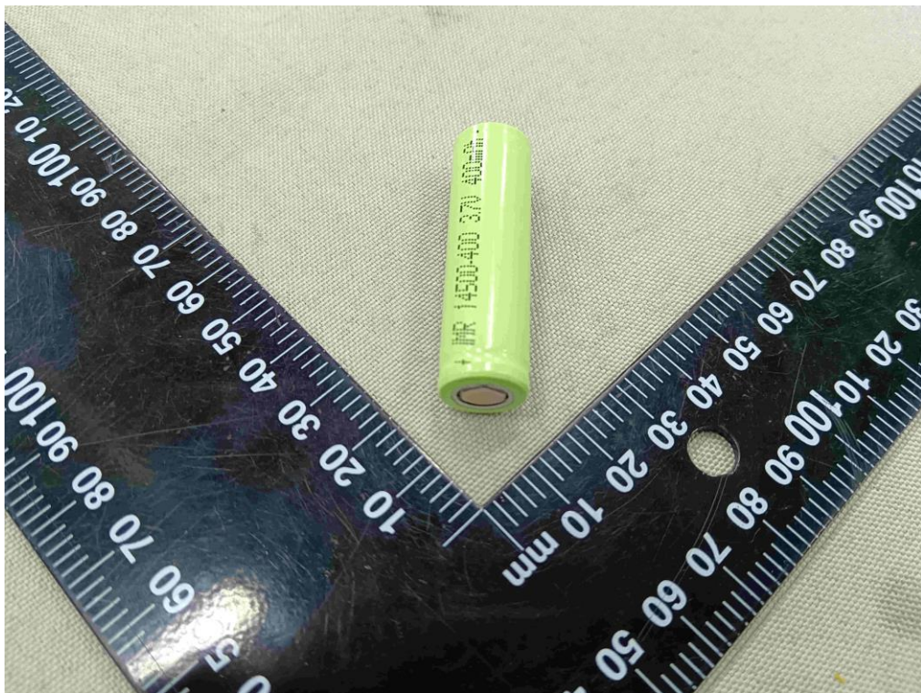
Figure 6 Side view of cell (model: IMR14500-400mAh)
