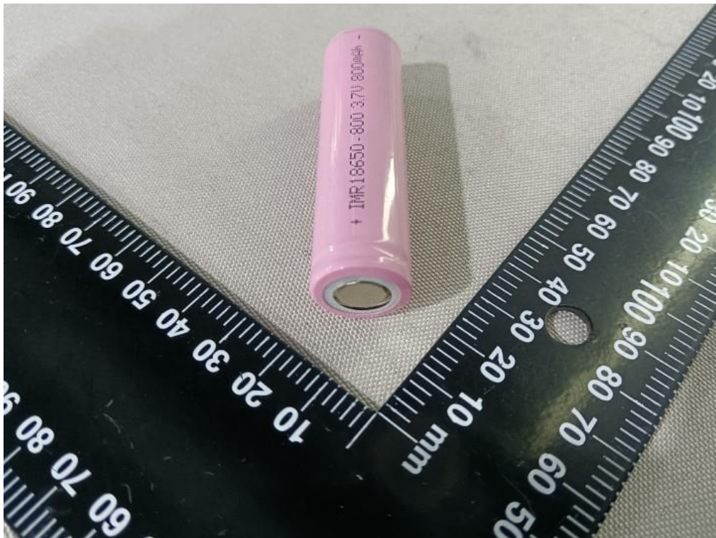
Figure 2 Side view of cell (model: IMR18650-800mAh)
