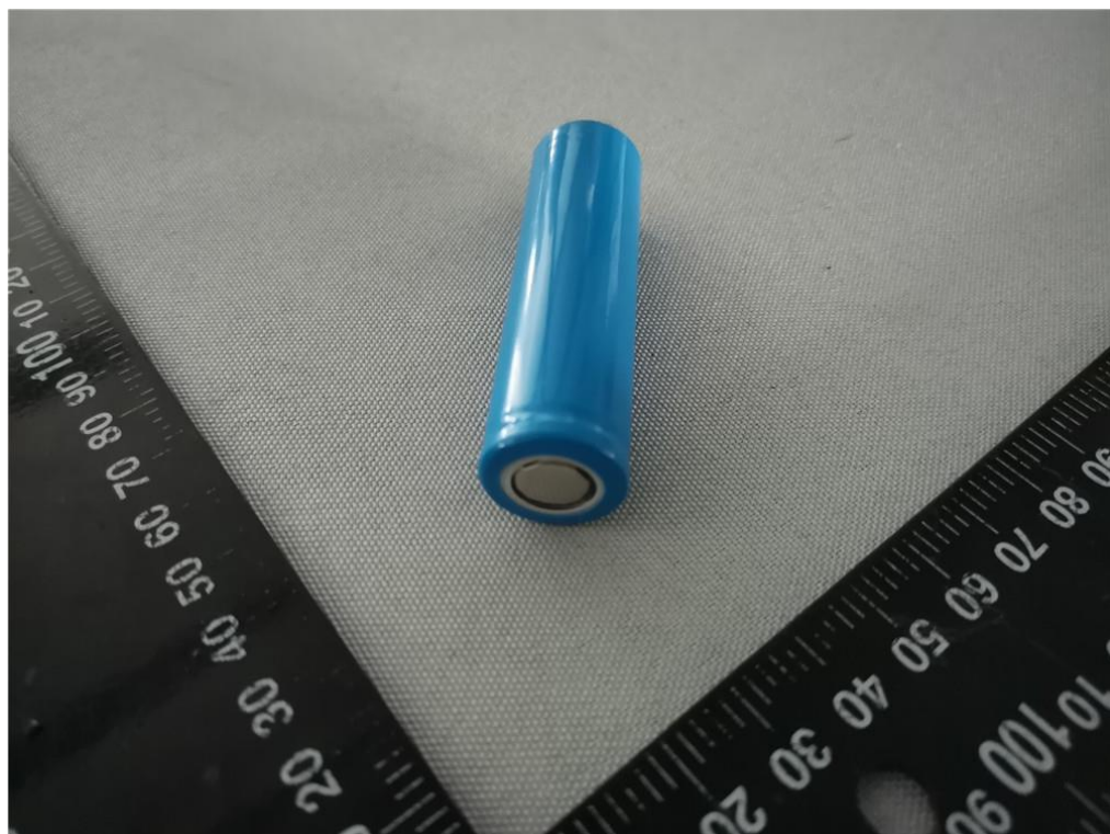
Figure 4 Side view of cell (model: IMR18650-1500mAh)
