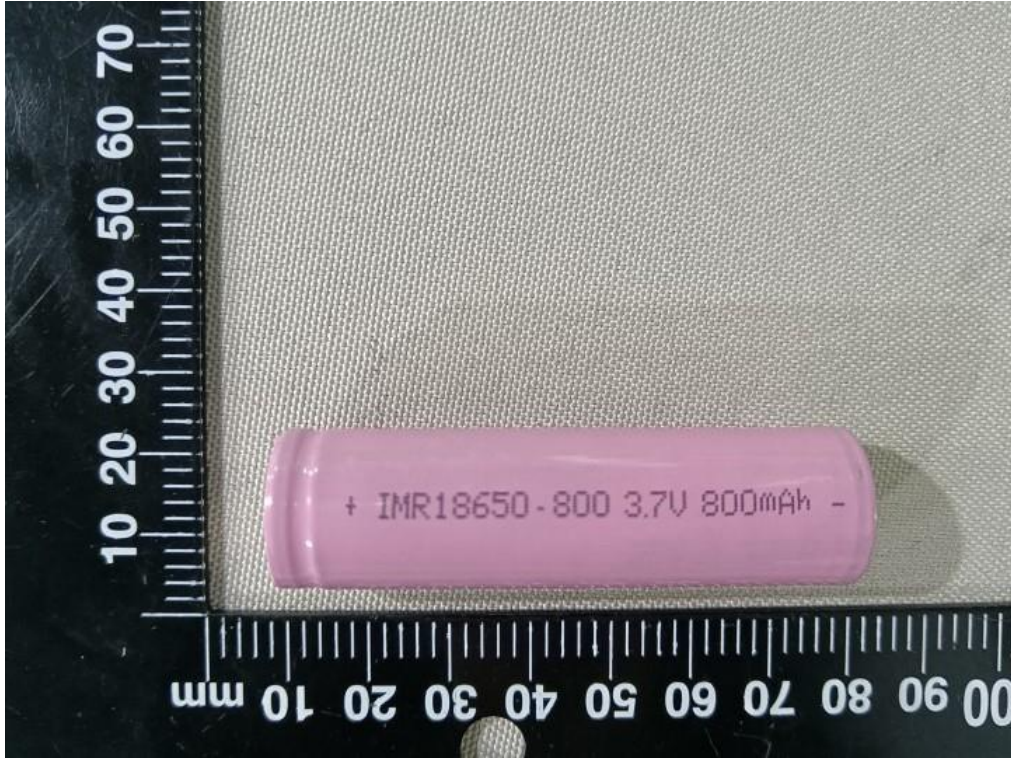
Figure 1 Front view of cell (model: IMR18650-800mAh)
