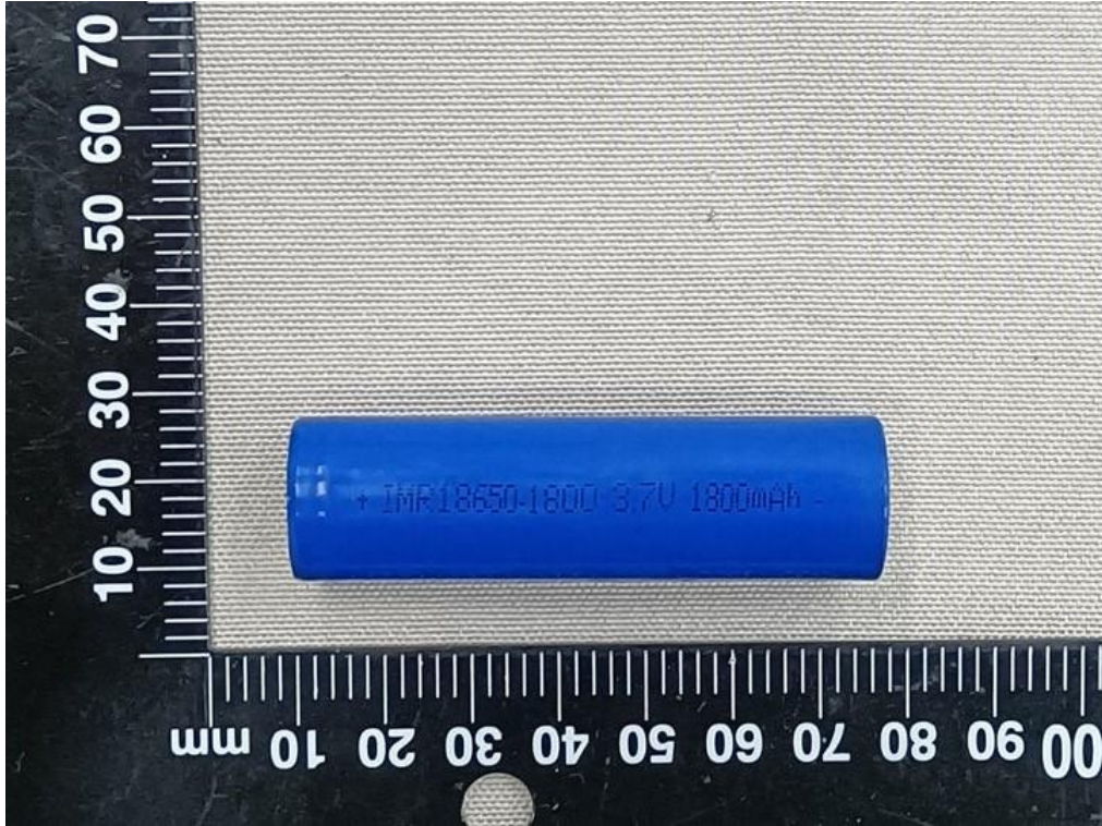
Figure 5 Front view of cell (model: IMR18650-1800mAh)
