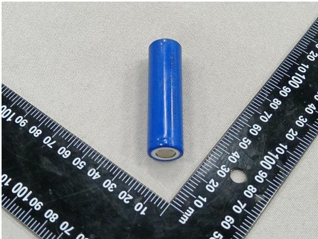
Figure 6 Side view of cell (model: IMR18650-1800mAh)
