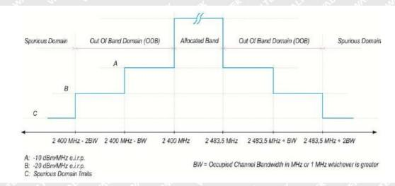
Within the 2400MHz to 2 483.5MHz band, the Out-of-band emissions are fulfilled by compliance with the Occupied Channel Bandwidth requirement.
