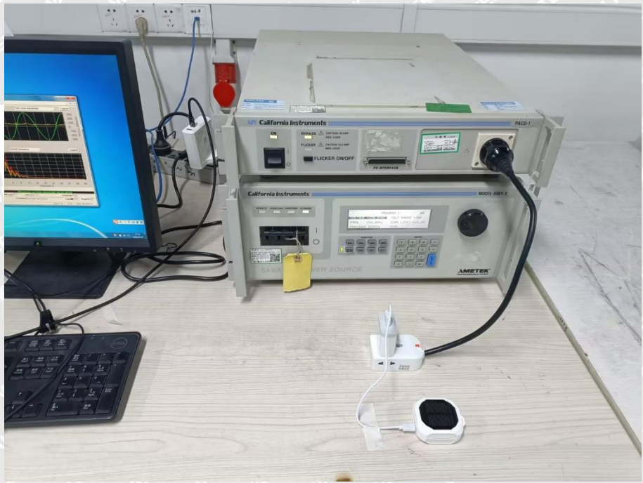
Harmonic/Flicker Test View
