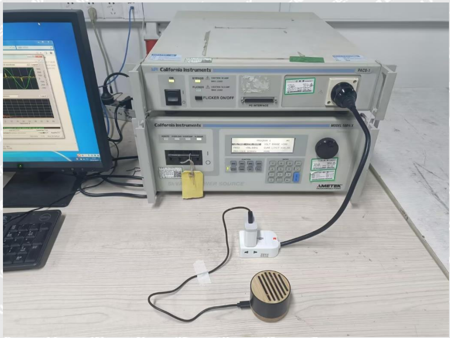
Harmonic/Flicker Test View
