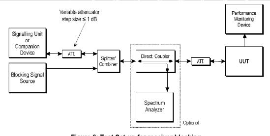
Figure 6: Test Set-up for receiver blocking
