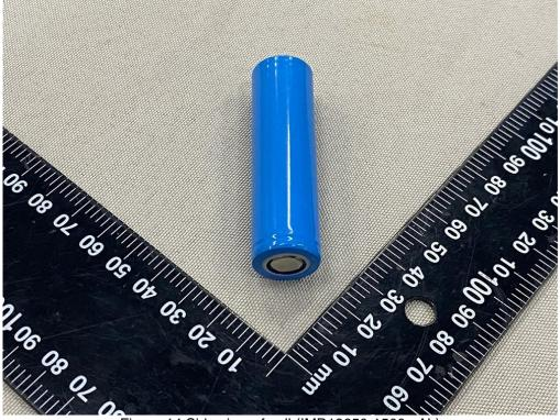
Figure 14 Side view of cell (IMR18650-1500mAh)
