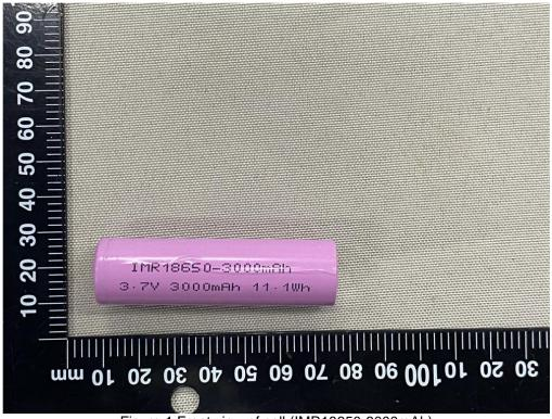
Figure 1 Front view of cell (IMR18650-3000mAh)
