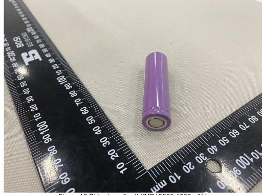
Figure 16 Side view of cell (IMR18650-1200mAh)
