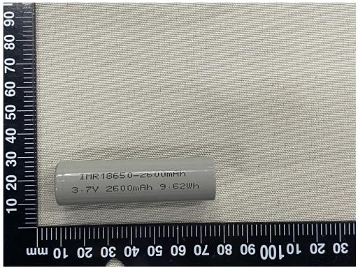
Figure 3 Front view of cell (IMR18650-2600mAh)
