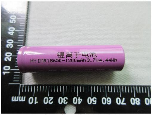
Figure 15 Front view of cell (IMR18650-1200mAh)
