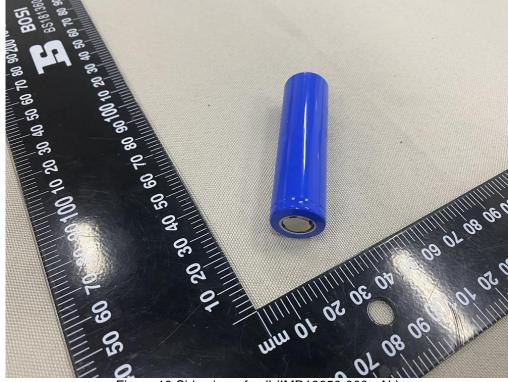
Figure 18 Side view of cell (IMR18650-800mAh)
