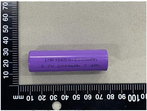
Figure 9 Front view of cell (IMR18650-2000mAh)
