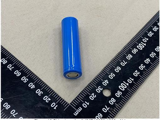
Figure 12 Side view of cell (IMR18650-1800mAh)
