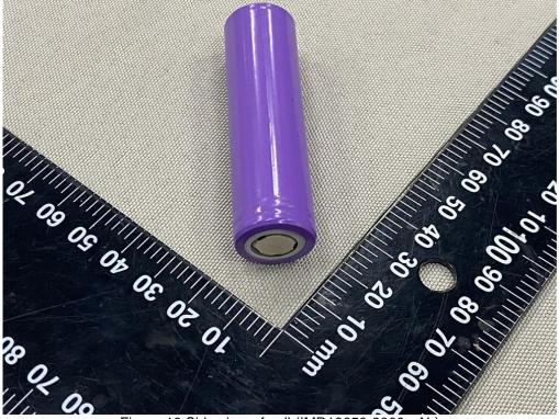
Figure 10 Side view of cell (IMR18650-2000mAh)
