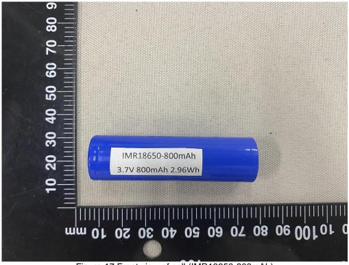
Figure 17 Front view of cell (IMR18650-800mAh)
