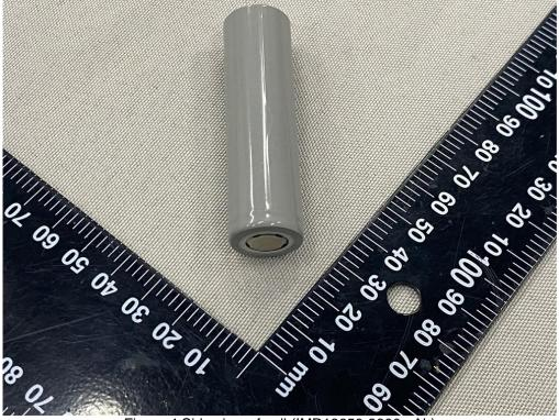
Figure 4 Side view of cell (IMR18650-2600mAh)
