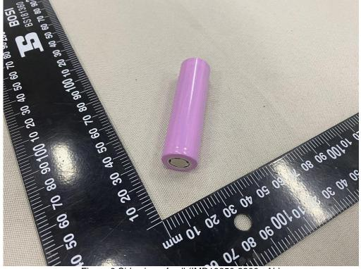
Figure 8 Side view of cell (IMR18650-2200mAh)
