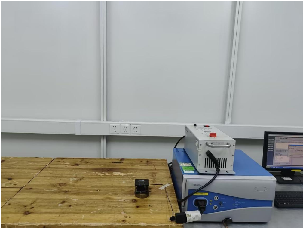
Fast transients/Surges/ Voltage dips at the AC mains power ports
