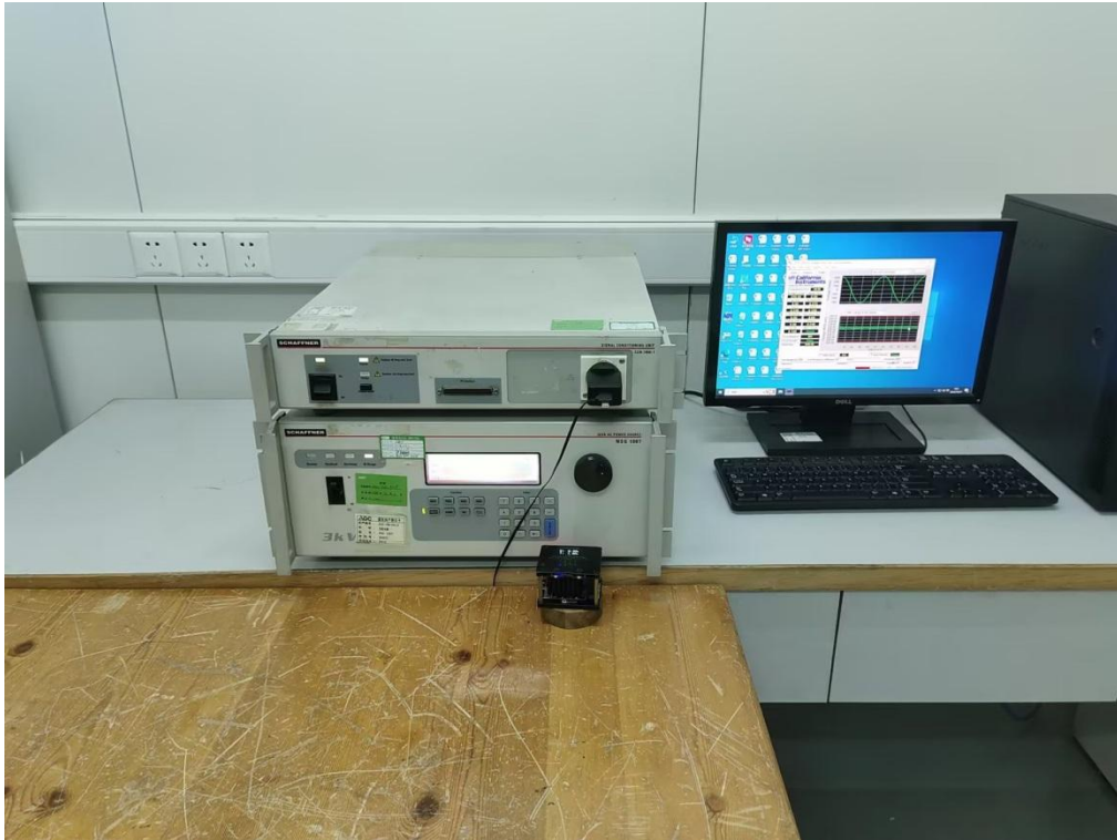
Harmonic current emissions & Voltage fluctuations and flicker
