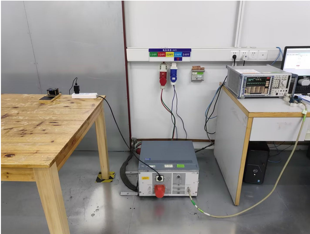
RADIATED EMISSION TEST SETUP (BELOW 1GHz)
