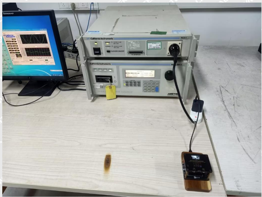
Harmonic/Flicker Test View
