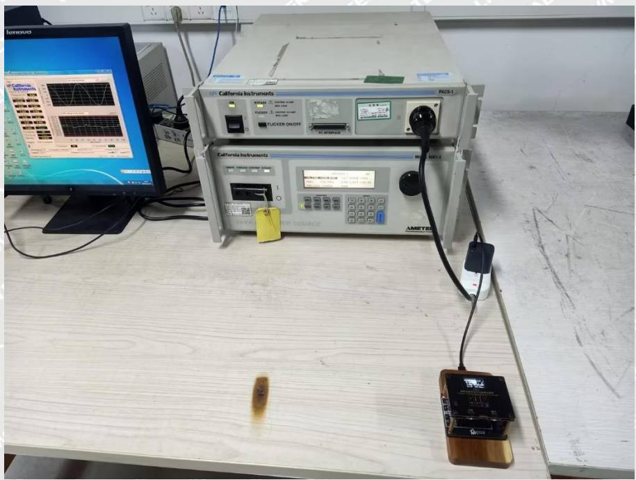
Harmonic/Flicker Test View
