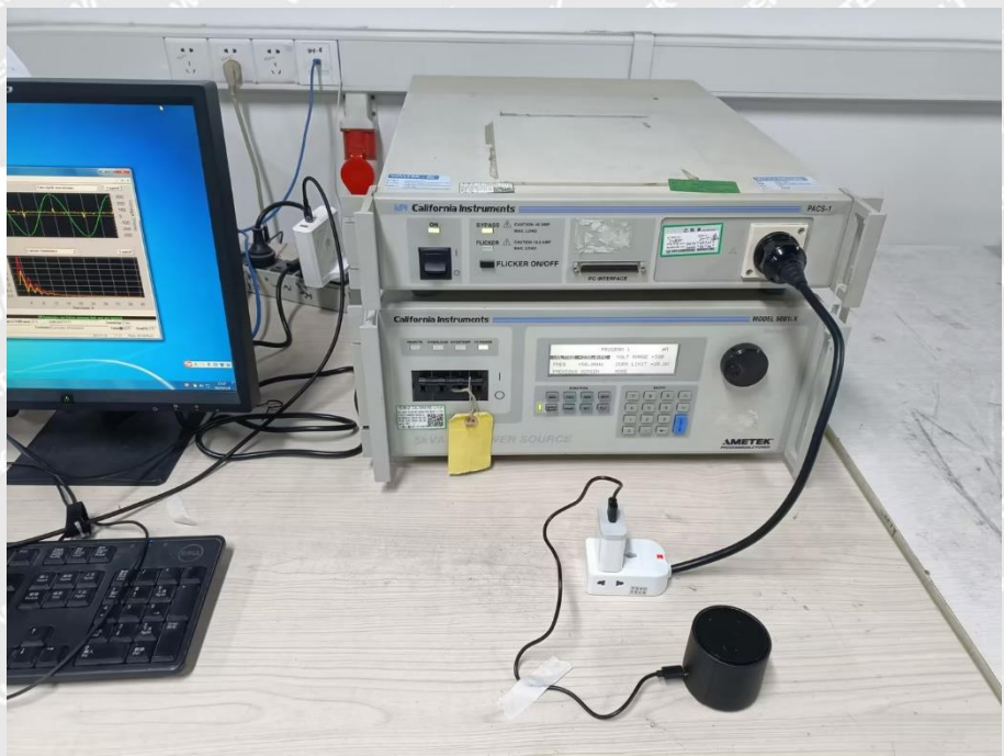
Harmonic/Flicker Test View
