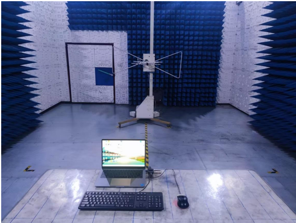
Radiated emissions at frequencies up to 1 GHz
