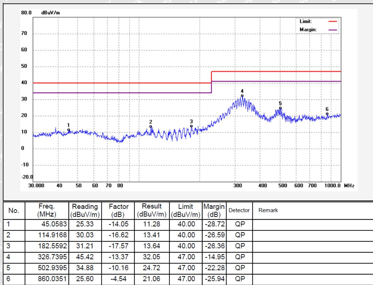
**Vertical Polarization (Discharging mode)**
