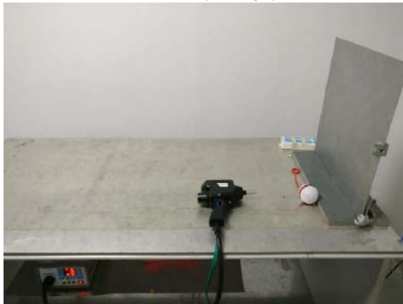
ESD Test Setup Photograph
